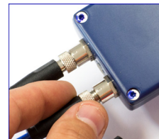
III. Manually unscrew connector
