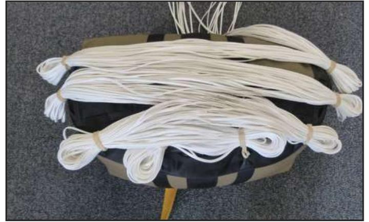
Continue the lines stowage on deployment bag and let a 60 cm length of lines free between the last stowage and top of risers.
