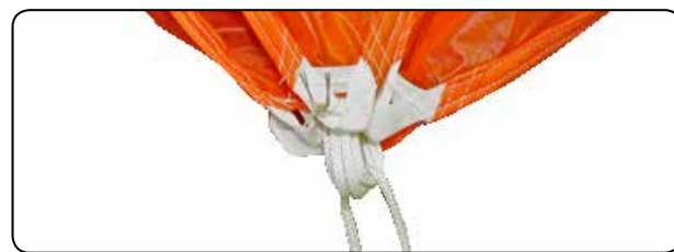
7.11 Tying the top tie-tabs.
