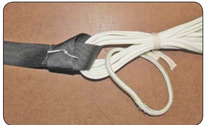
8.1 Bridle installation onto the apex.
