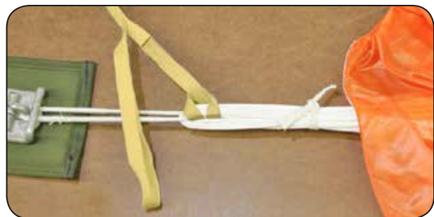
7.2 Installing the zip-strip to the apex.
