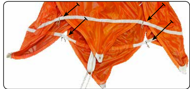
7.10 Tying the center tie-tabs.
