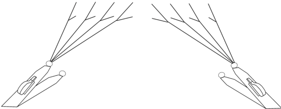
Figure 3: Correct attachment of the rear line set to the rear risers
