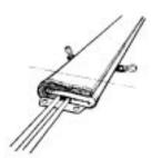
• Fold the periphery over so that the grommets are level with the \*Nitrile Rubber 'O' Rings on the mouth lock. See Fig. below:
