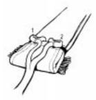
• Use regular rubber bands to stow the left and right line groups together as shown in Fig. below:
