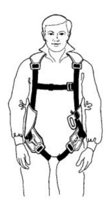
The chest strap should be positioned at mid-chest level.
