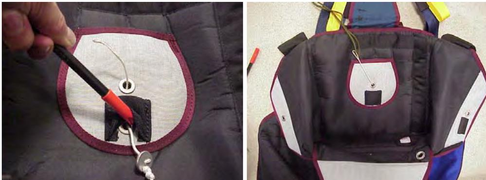
Place the risers on the sides of the harness/container and insert the bag into the reserve container. Using the "T" tool, pass the pull-up chord through the grommets of the deployment bag.
