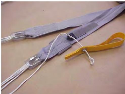
Pass the extreme of the control line through the grommet of the steering toggle, from the rear to the front. Pass the lower part of the toggle through the control line loop of the extreme.
