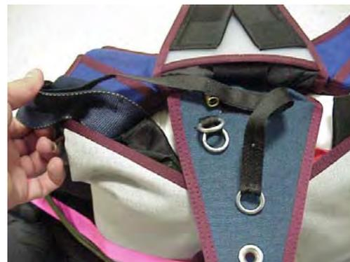
Once the reserve parachute is packed and introduced into the reserve container, before closing the container, the reserve ripcord cable must be passed through the ring of the RSL, and in between the two rings of the reserve closing flap.
