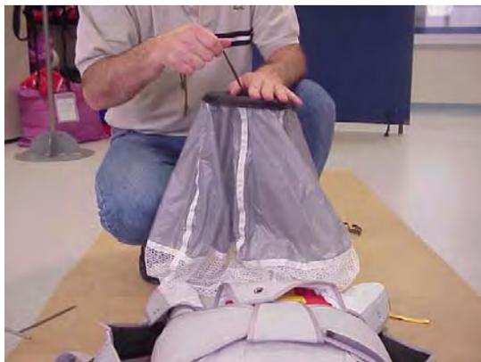
Compress the pilot chute and lock it with the spare locking pin. Pull out the pilot chute fabric from the spring to avoid being trapped.
