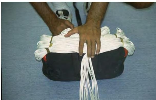
Pull the pilot chute bridle to check that the connection ring of the canopy is not trapping canopy fabric and it is stopped inside the deployment bag by the grommet.
