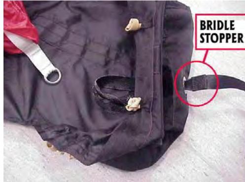
2.- Pass the free loop Nr. 2 of the pilot chute bridle through the connection ring of the main canopy. Next pass the connected pilot chute and deployment bag through this loop.
