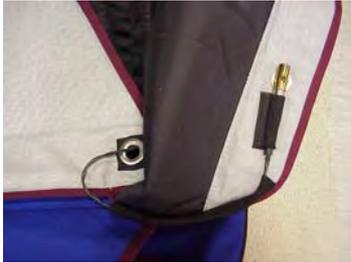
The release unit (EOS) cable should be routed via flap Nr. 1 and 2.
