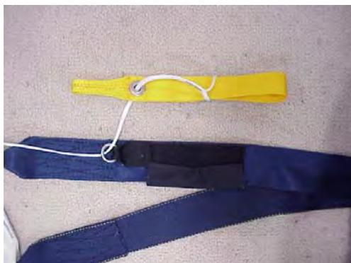
Move the loop along the toggle up to the grommet of the toggle. Pull to fix. Attach the toggle to the velcro on the riser.
