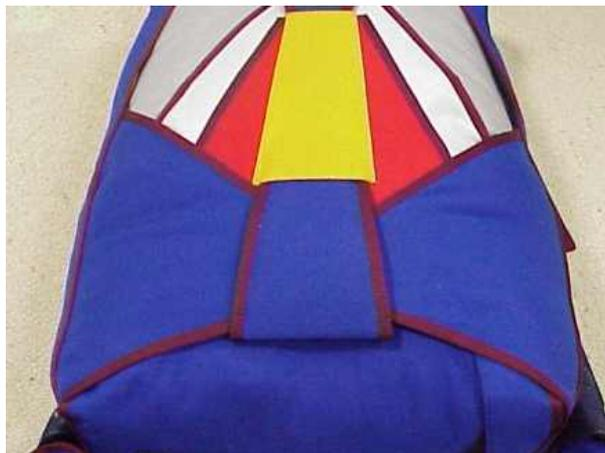
Inspect the risers so that they are properly tied and close the riser covers. Be sure to introduce the riser cover flaps into the corresponding pouches, under main and reserve risers.
