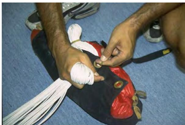
The loop of the suspension lines stow must not exceed 4 cm (1 3/4") from the elastic rubber band.
