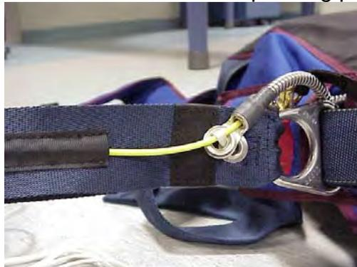
Attach the cut-away grip to the Velcro in the harness.
