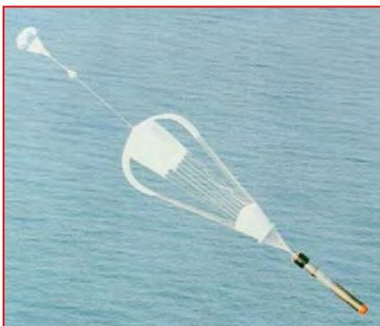
CIMSA Ingeniería de Sistemas, S.A. designs and produces bomb and torpedoes stabilisation systems, like the various models for the MU-90 vessel, plane and helicopter torpedoes.
