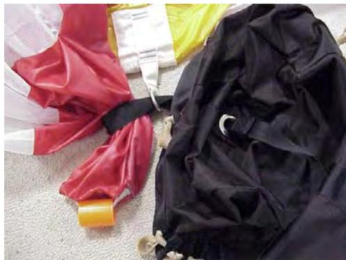
3.- Pull to fix, being careful to avoid friction of pilot chute bridle with union bands/chords when fixing the knot.
