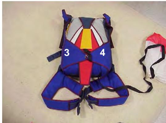
3.- Fasten the Velcro of the pilot chute bridle to the closed upper flap. Introduce the curved locking pin in the closing loop. Remove pull-up chord.
