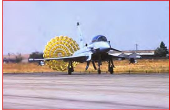
The use of this braking parachute system provides a serious reduction in operational and overhaul costs, as well as shortest landing distances, increase of the plane's life cycle and increase of safety in wet and icy landing ways.
