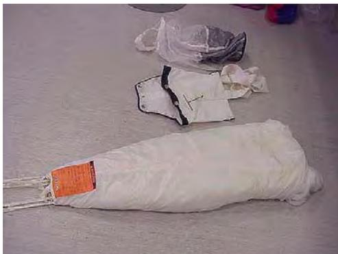
Place yourself on the side of the canopy. Put one hand under the slider and the other one over the bundle. “S” fold it and check that suspension lines remain tense during this operation.
