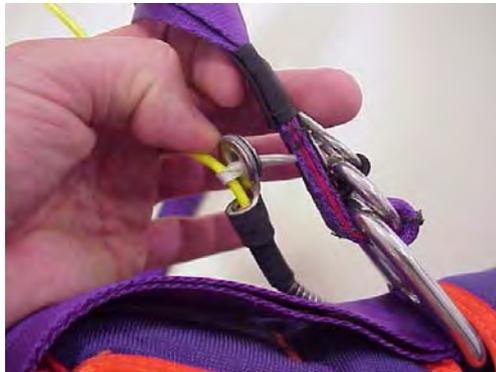
Introduce the extreme of the cable into the corresponding pouch of the rear riser.
