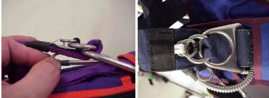
Pass the loop through the grommet of the cut away cable housing. Pass the yellow cable through the loop.
