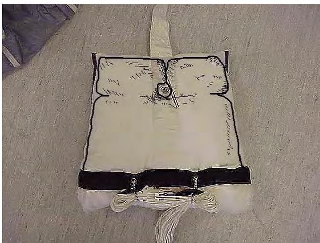
Close the flap of the deployment bag by passing the elastic bands through the grommets. Lock it by stowing the suspension lines in both elastic bands.
