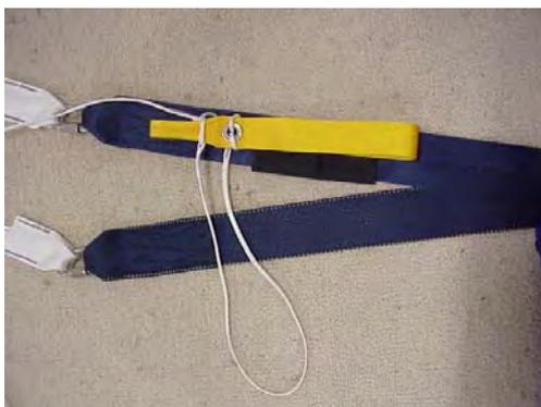
2.- Insert the upper part of the toggle through the brake locking loop and, once inserted, fit the toggle upper and lower part into the pouches above and below the guiding ring. Pull the control line until the toggle is in touch with the guide ring.
