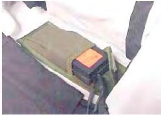
Position the processing unit into the elastic pouch on the bottom of reserve container, so that the spare cable pocket is to the right.
