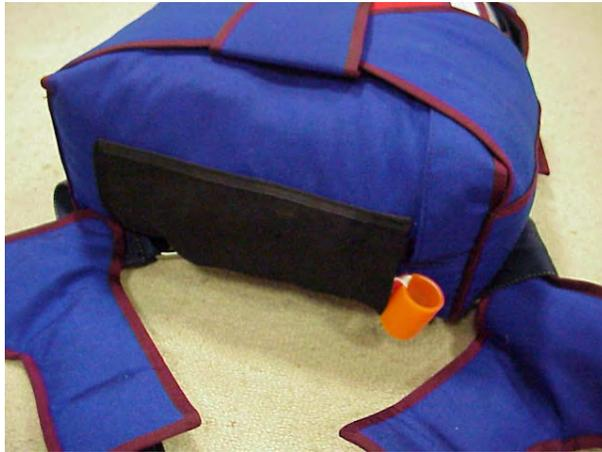
Close the locking pin protection flap of the main container.
