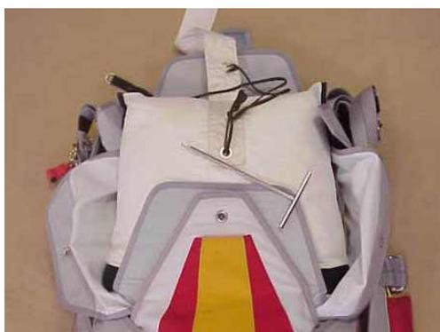
Close lower flap Nr. 1 by passing the pull-up chord. Use a spare locking pin to maintain the position.
