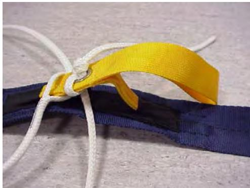
3.- "S" fold the remaining of the control line inside the elastic pouch placed under the same rear riser.
