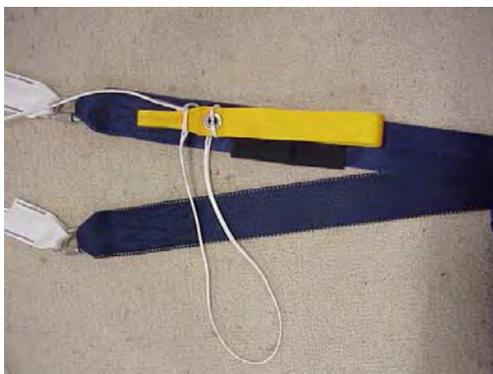
3.- "S" fold the remaining of the control line inside the side cover.
