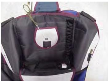
Align the release unit (EOS) so that it lies parallel to the long axis of the container, ensuring that the loop hole is in line with the right hand inner edge of the grommet.
