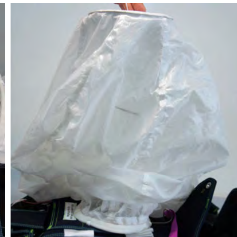
27. Pass the pull up cord cleanly through the pilot chute from bottom to top plate.
