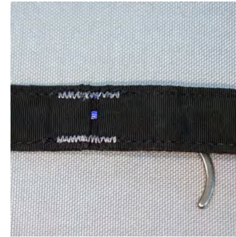
13. Make sure coloured mark shows at the bottom of the bridle window.
