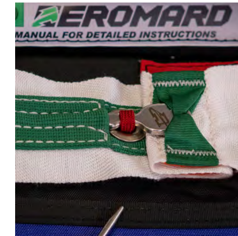
20. Insert reserve bridle Bulge Pin through red lanyard loop and green pin housing while seating magnets. Ensure red loop has passed the bulge of the pin.
