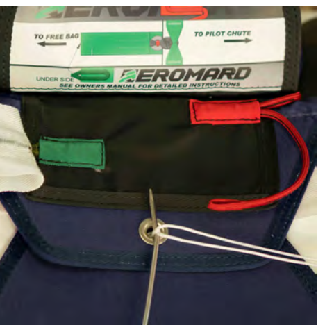
18. Feed the red MARD Lanyard into the red tuck tab. Leave 3 inches excess red lanyard.
