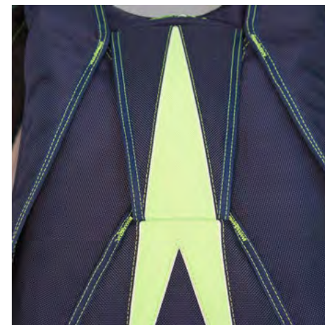
33. Close the final cover flap and tuck the tabs under the #6 flap.
