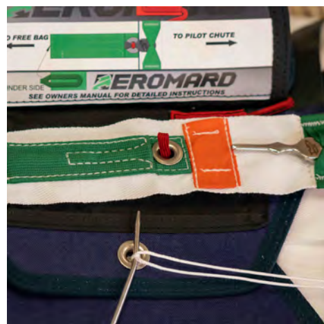
19. Lay the bridle over flap #2, routing the red MARD lanyard loop through the bridle grommet from bottom to top.
