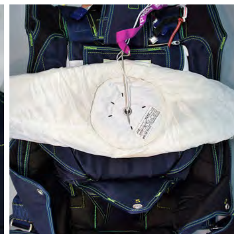
29. Press the pilot chute down into position and hold with a temporary pin. Make sure not to catch the pilot chute fabric under the plate or between the spring coils.
