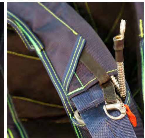
4. RSL Prepared and ready for connection to Riser.
