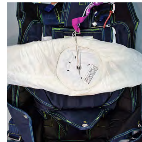
24. Press the pilot chute down into position and hold with a temporary pin. Make sure not to catch the pilot chute fabric under the plate or between the spring coils.
