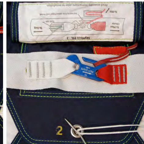
24. Lay the Skyhook bridle over flap #2. Attach the red lanyard to the Skyhook.
