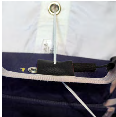
13. To ensure proper AAD activation make sure your reserve loop is threaded through the AAD cutter.
