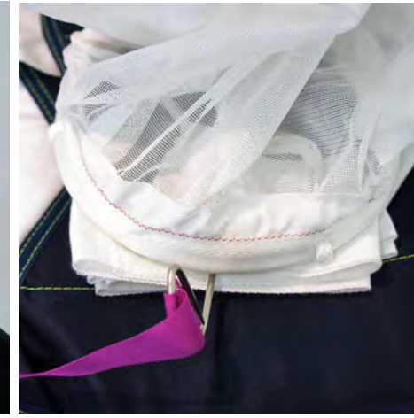
23. Ensure the lower spring coil is up against the spring ejector plate and that the excess bridle sits under the pilot chute without catching the fabric under the spring.
