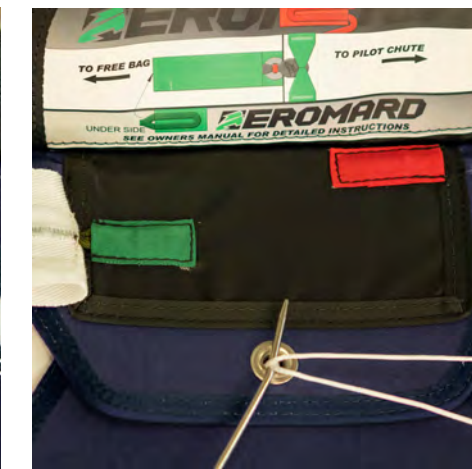
17. Insert the green loop into the green tuck tab.
