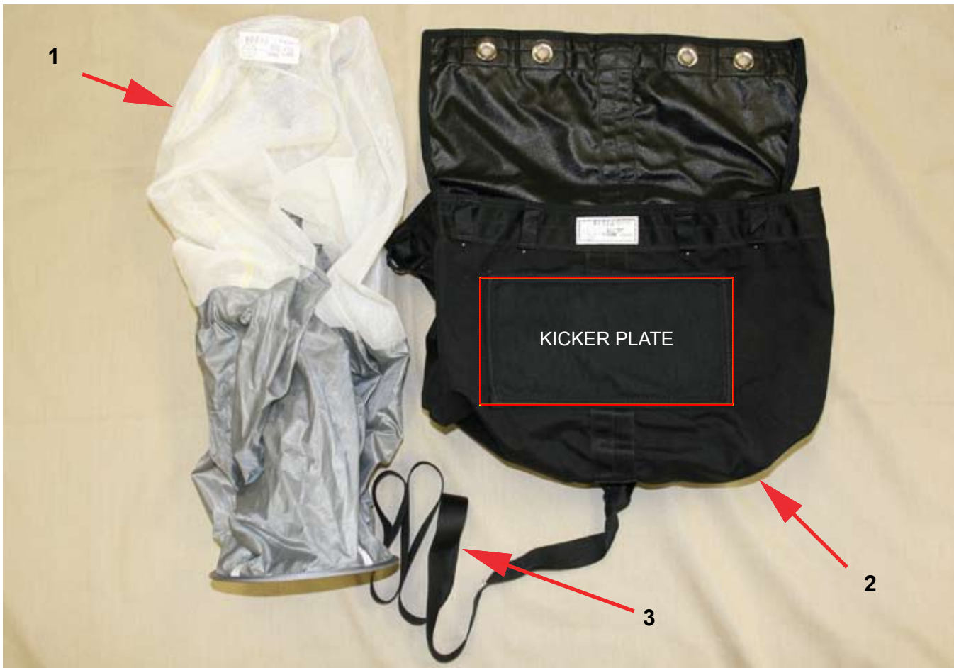
Figure 6. MJ-10 Main Deployment Bag Assembly
