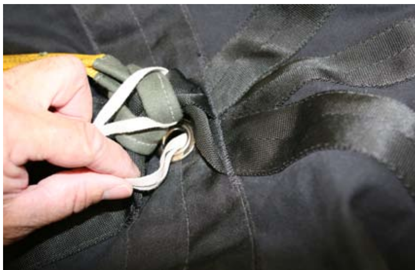
Figure 5-74. Place 80-Pound Break Cord Through Grommet
