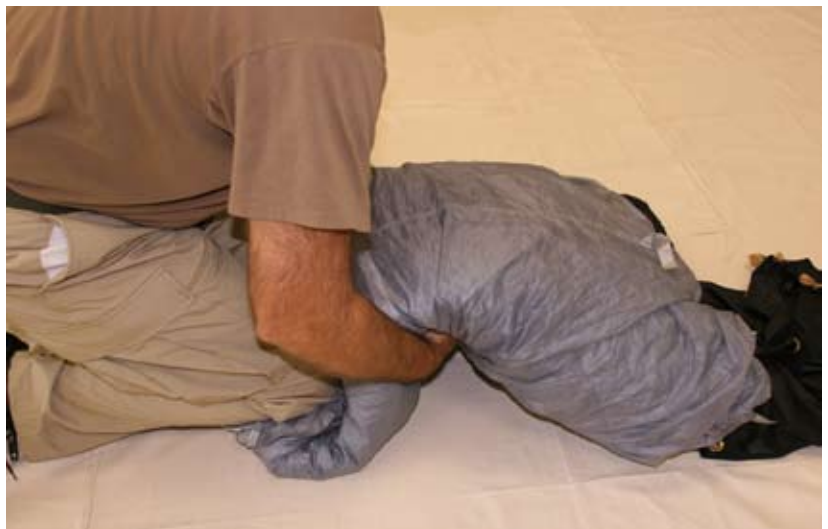
Figure 5-21. “S” Fold The Parachute
