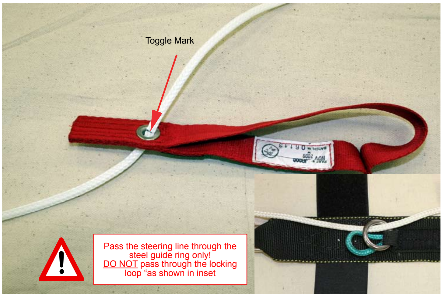
Figure 2-18. Thread Steering Line Through Steel Ring And Toggle Grommet
