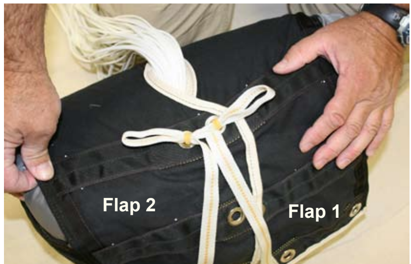
Figure 5-66. Make The Second Bridle Bight
