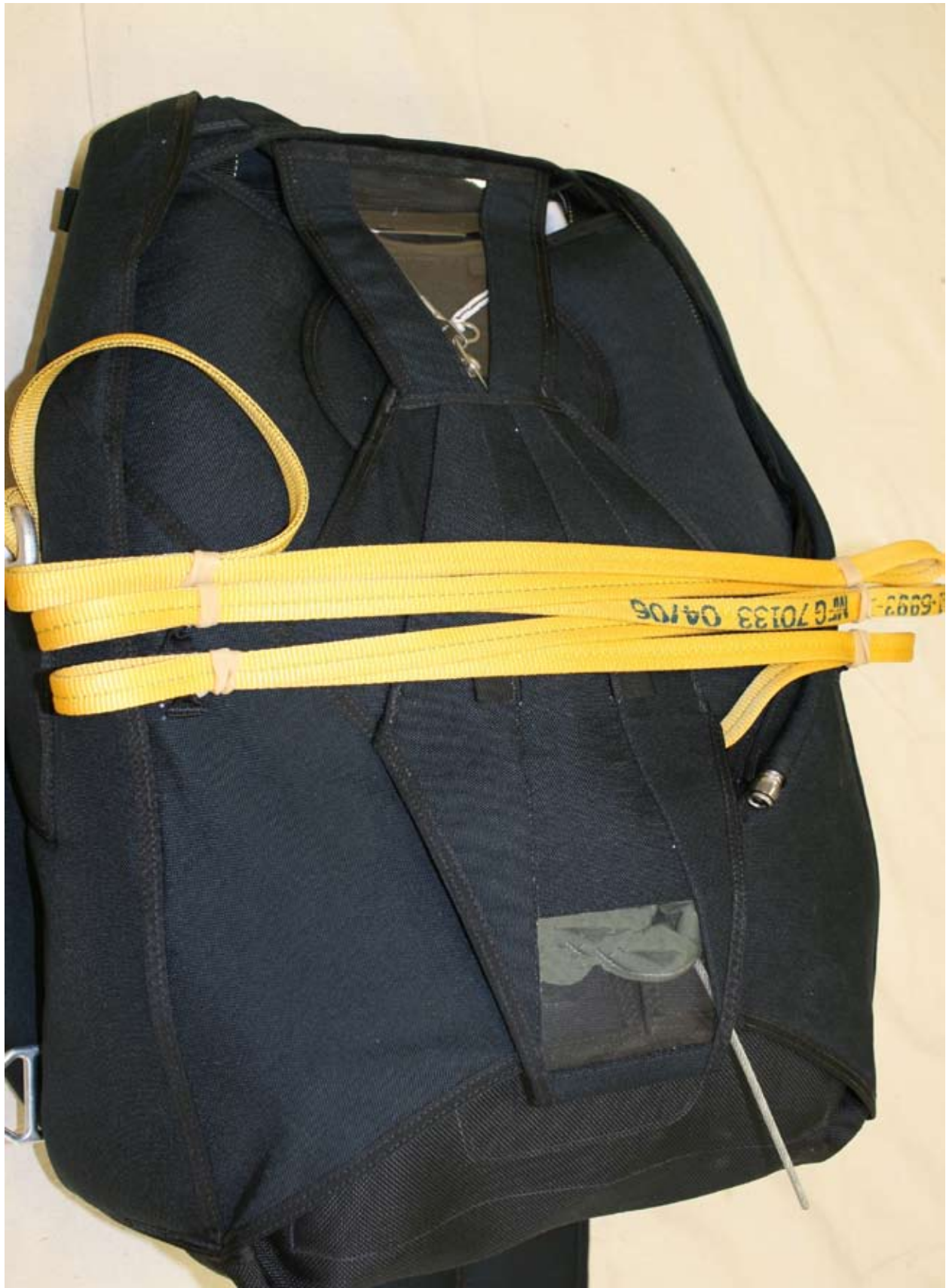
Figure 5-95. Completed Dual Bag Static Line Configuration
