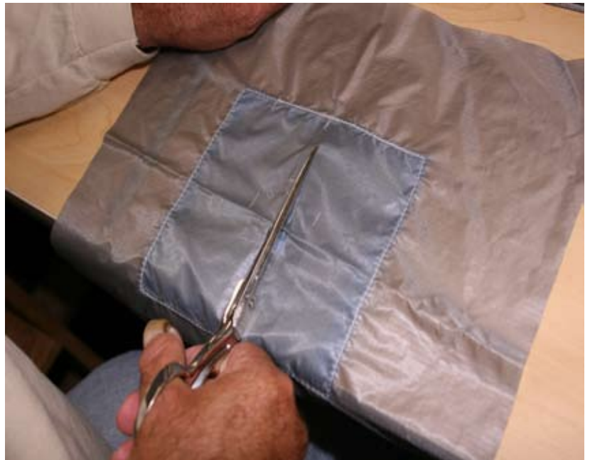
Figure 7-8. Begin Removing Damaged Material
