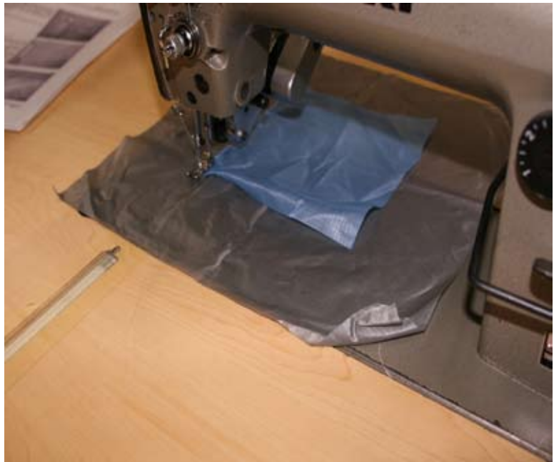
Figure 7-6. First Two Corners Sewn Down
