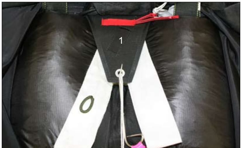
Figure 2-150. Pin The Closing Loop Above Flap 1
