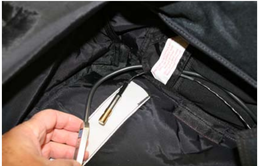
Figure 2- 4. CYPRES Cable Routing
