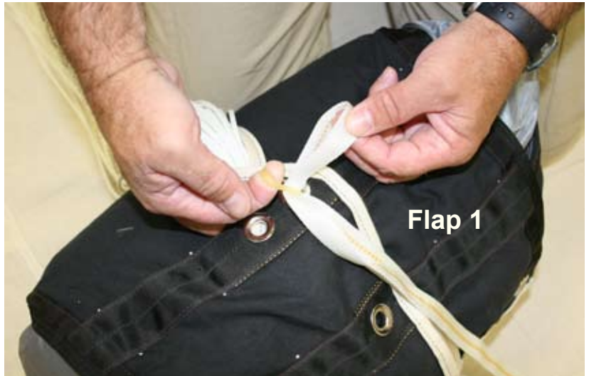
Figure 5-63. Secure First Bridle Bight
