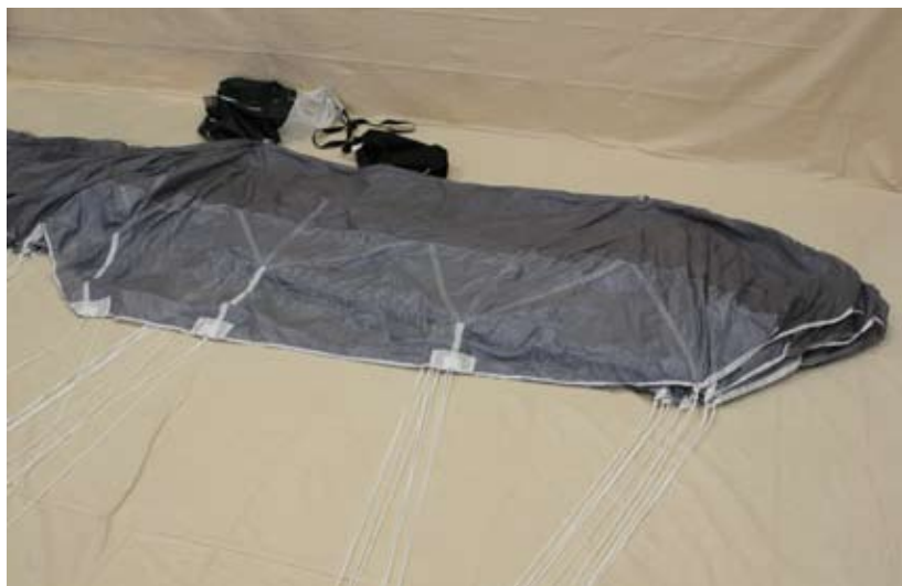
Figure 5-5. Clear The Nose Cells
