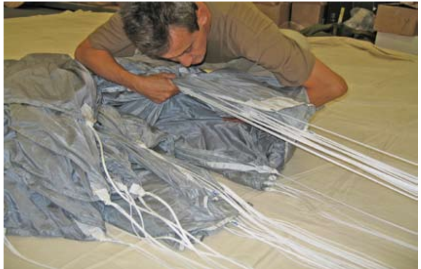
Figure 2-57. Clear Fabric Between Line Groups A & B
