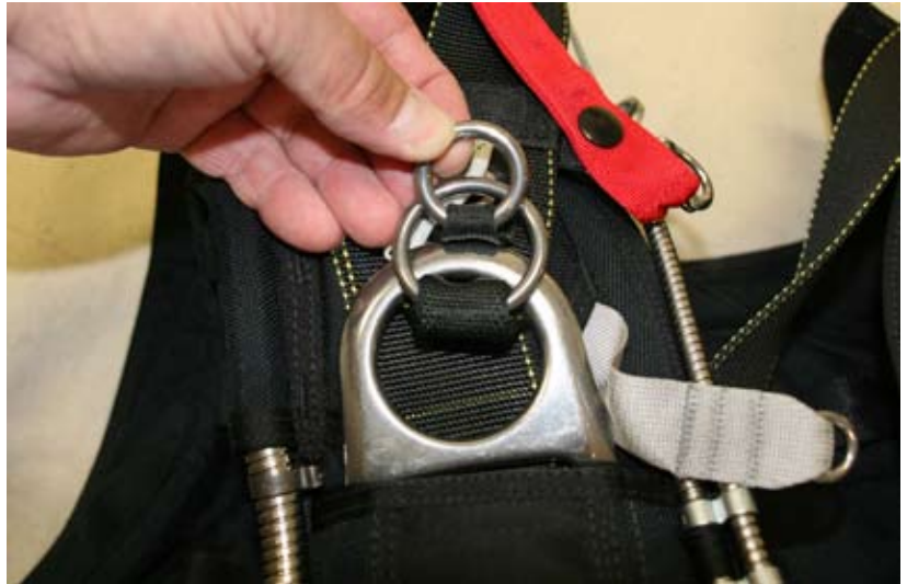
Figure 3-2. Insert Third Ring
