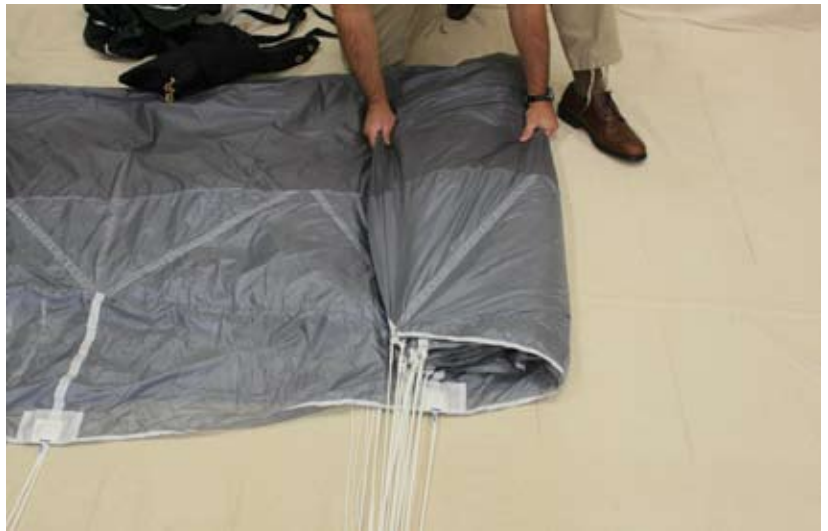
Figure 5-7. Fold The A Line Group Onto The B Line Group
