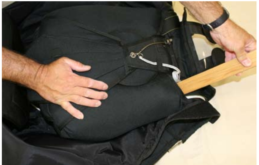
Figure 2-143. Carefully Tuck In The Reserve Tuck Tabs
