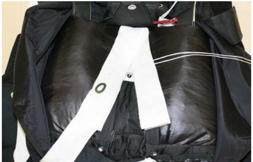
Figure 2-149. "S" Fold The Bridle Material
