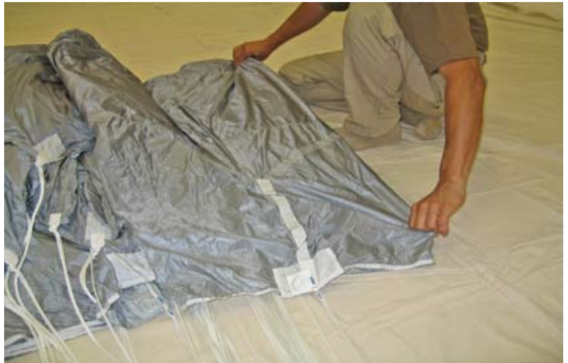
Figure 2-63. Neaten The C-D Fabric Fold
