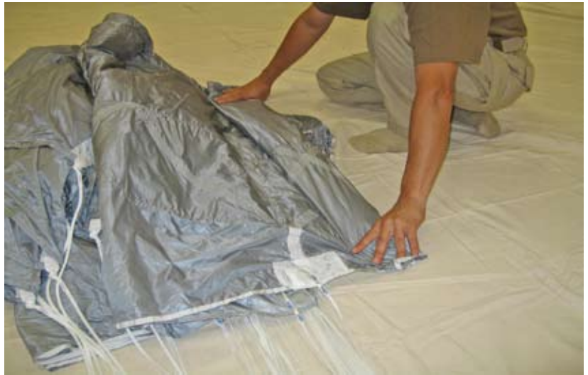
Figure 2-62. Long Fold The A-B Fabric Fold
