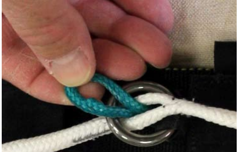
Figure 2-37. Pull The Locking Loop Through Cat-Eye
