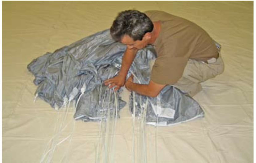
Figure 2-54. Separate The Left & Right Line Groups
