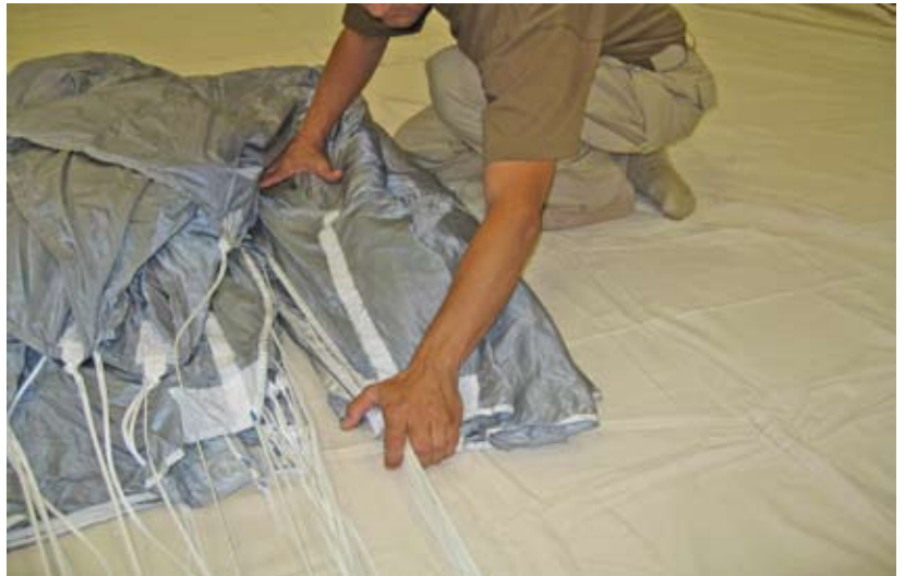
Figure 2-65. Clear The Stabilizer Panel
