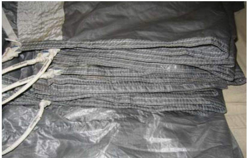
Figure 2-67. Close Up Of The Flaked Trailing Edge
