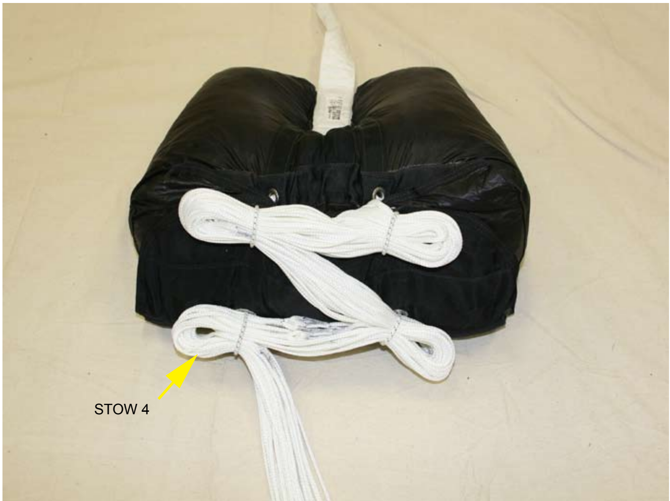
Figure 2-117. Place The Final Safety Stow
