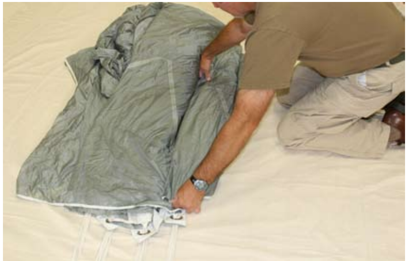
Figure 2-88. Long Fold The Fabric
