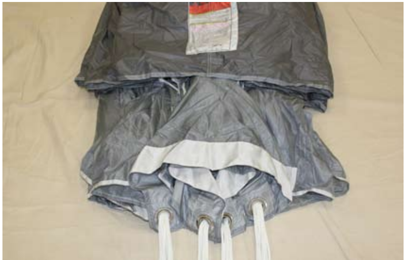
Figure 5-54. Set the Slider Back In Place
