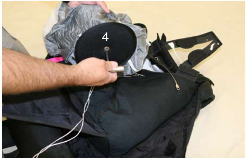
Figure 2-129. Place A Bodkin Into The Top Grommet
