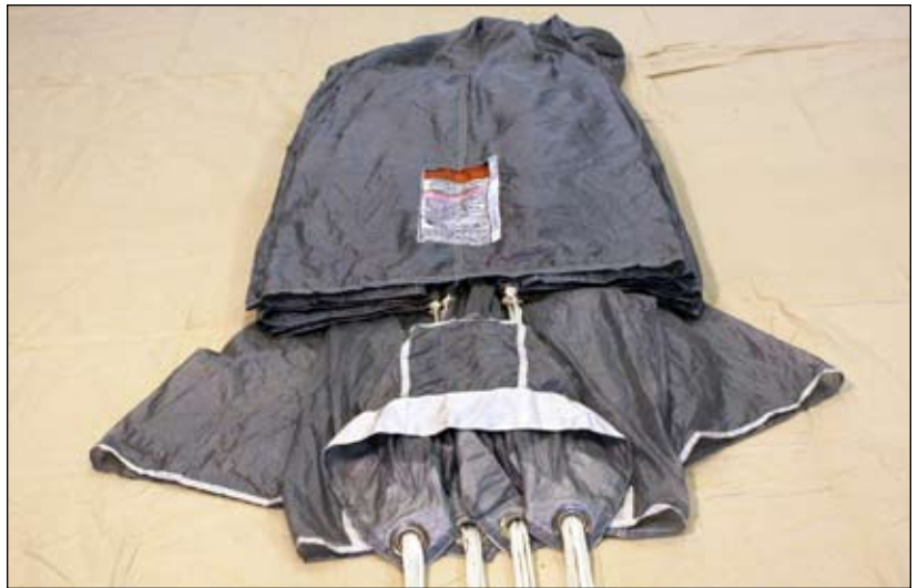
Figure 2-71. Raise The Slider Grommets To Slider Stops
