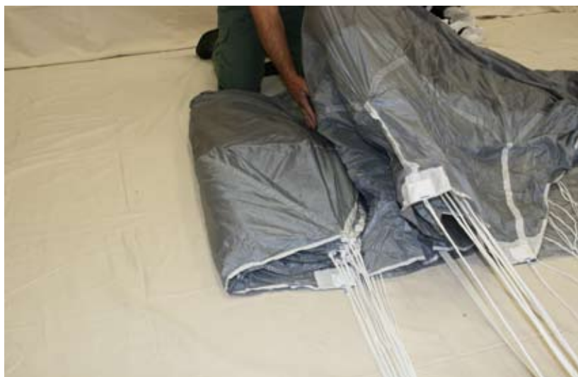
Figure 5-47. Fold The C Line Group Onto The A & B Groups
