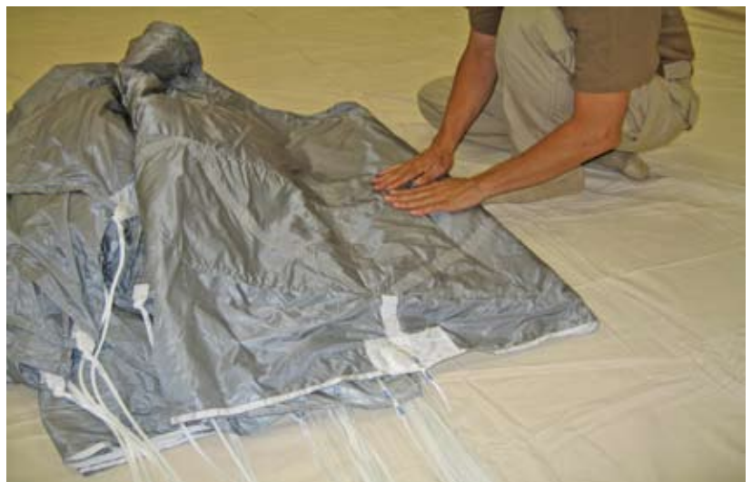
Figure 2-61. Neaten The A-B Fabric Fold
