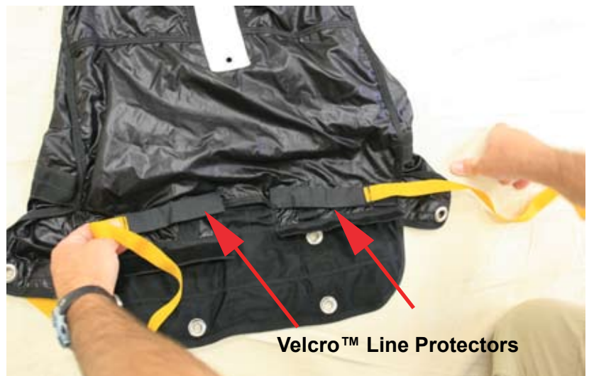
Figure 2-100. Install Velcro™ Line Protectors
