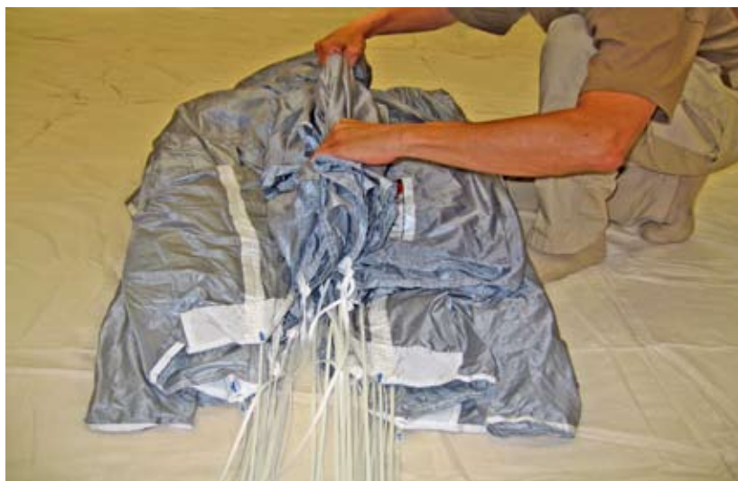
Figure 2-69. Lay Half The Flaked Tail Over
