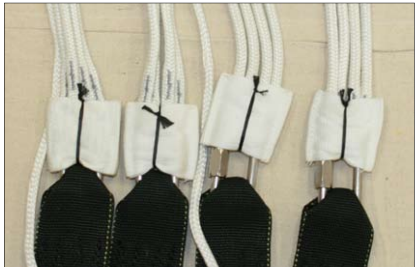
Figure 2-17. Link Protectors Installed
