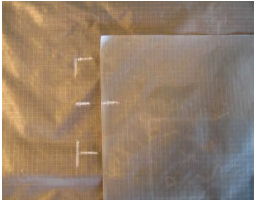
Figure 7-3. Mark The Repair Starting Point
