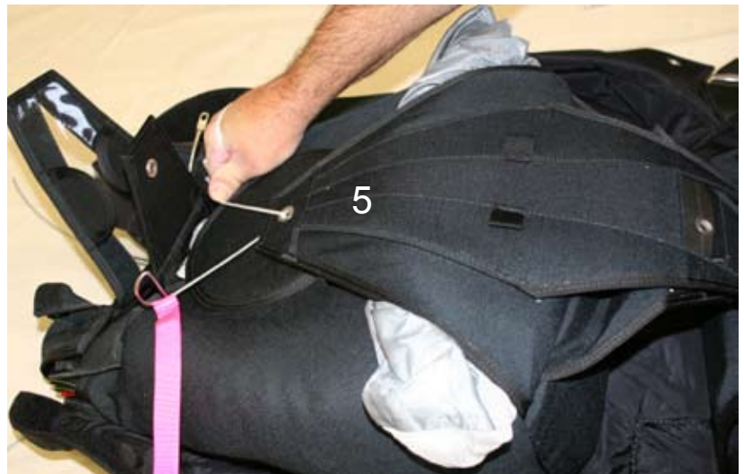
Figure 2-137. Divide The Remaining Pilot Chute Fabric
