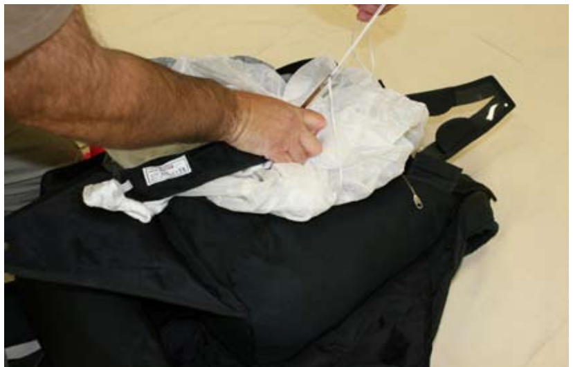
Figure 2-130. Run The Bodkin Through To The Bottom
