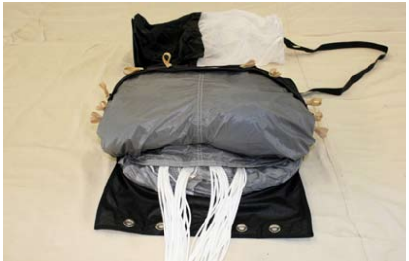
Figure 5-24. Ready For The Locking Stows
