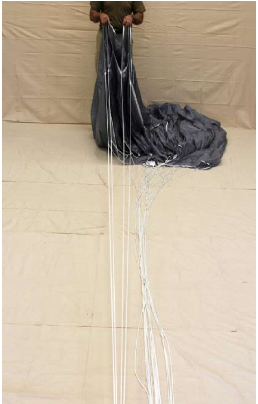
Figure 2-35. Check “A line” Continuity
