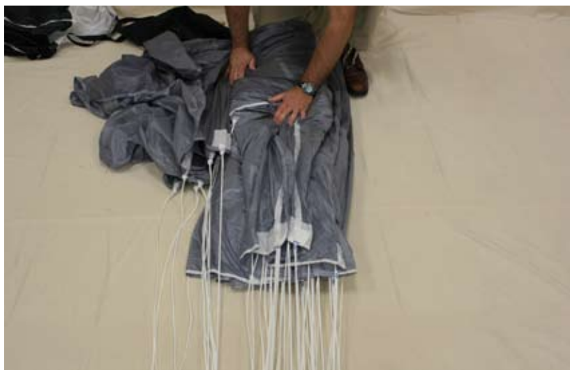
Figure 5-10. Fold The D Line Group Onto The C Line Group
