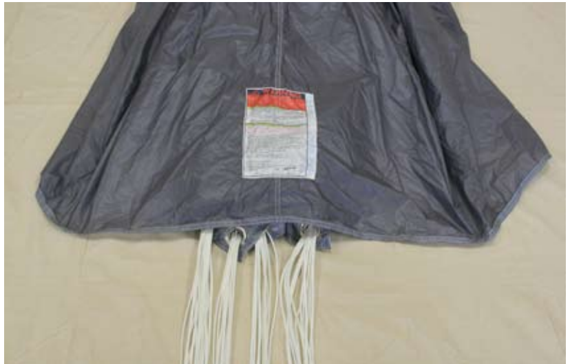
Figure 5-55. Lower Trailing Edge Just Below The Slider
