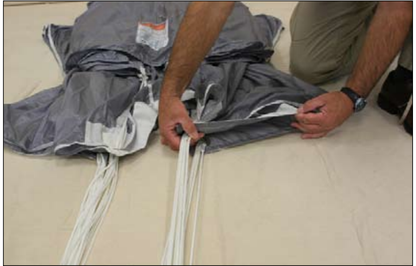
Figure 2-72. Quarter The Slider
