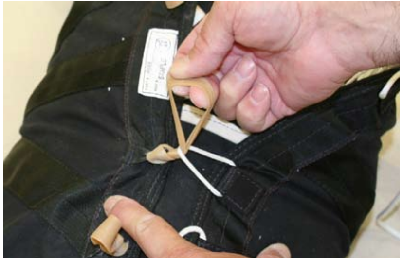
Figure 5-83. Start with Either Center Locking Band
