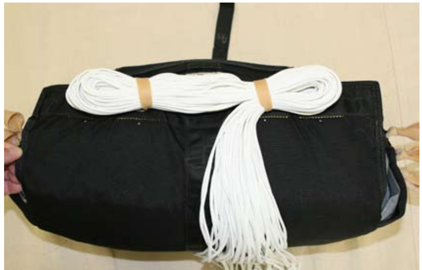
Figure 5-26. Place The Second Locking Stow
