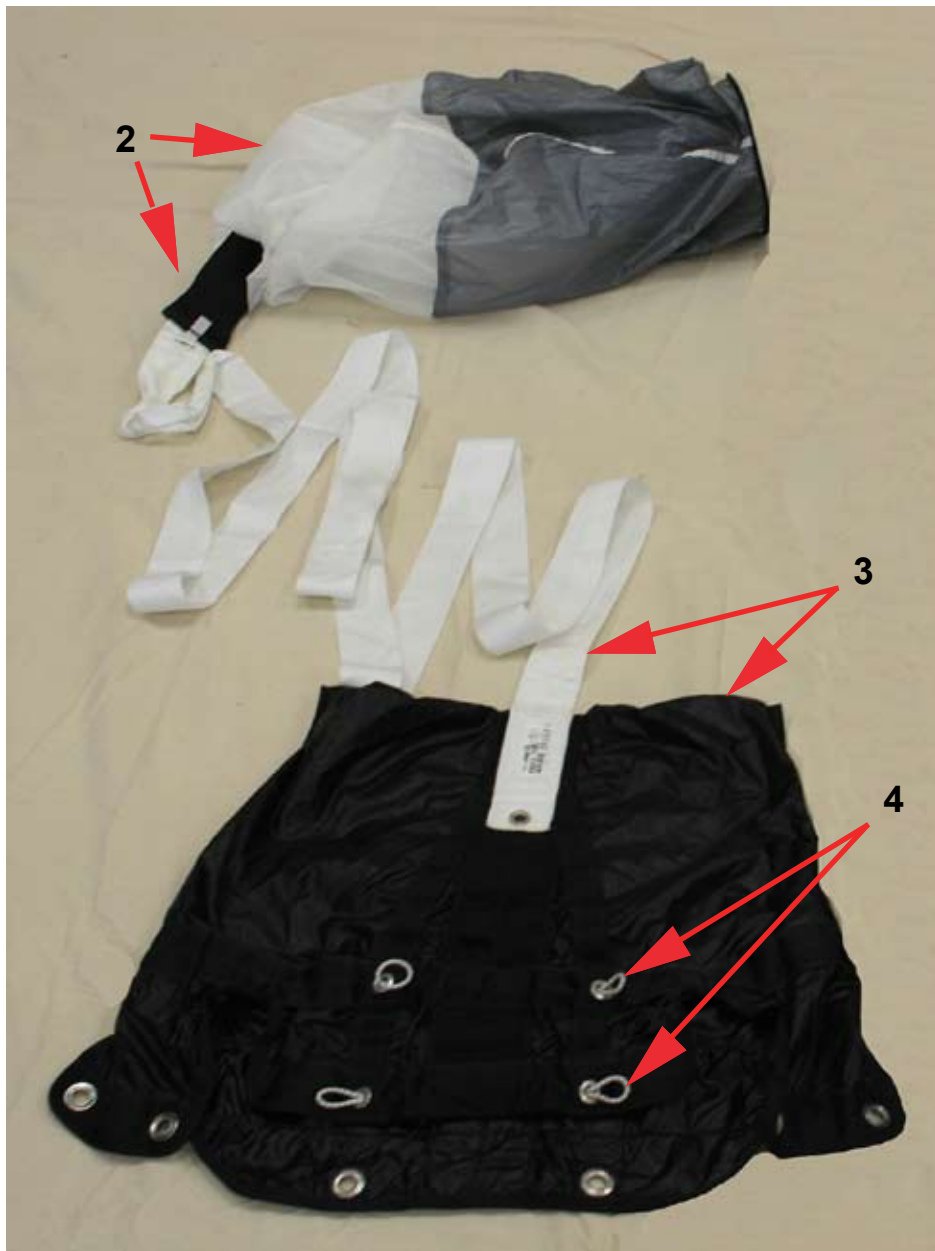
Figure 8. Dual Speed Reserve Deployment System
