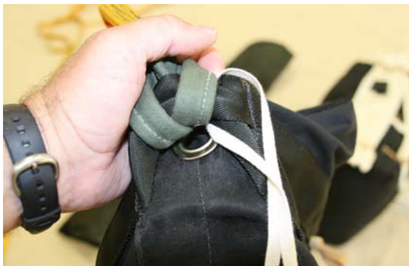
Figure 5-73. 80-Pound Break Cord Under Static Line Attachment
