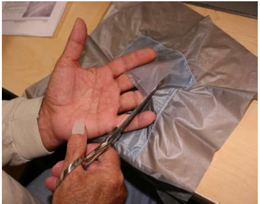
Figure 7-9. Complete Removal Of Damaged Material
