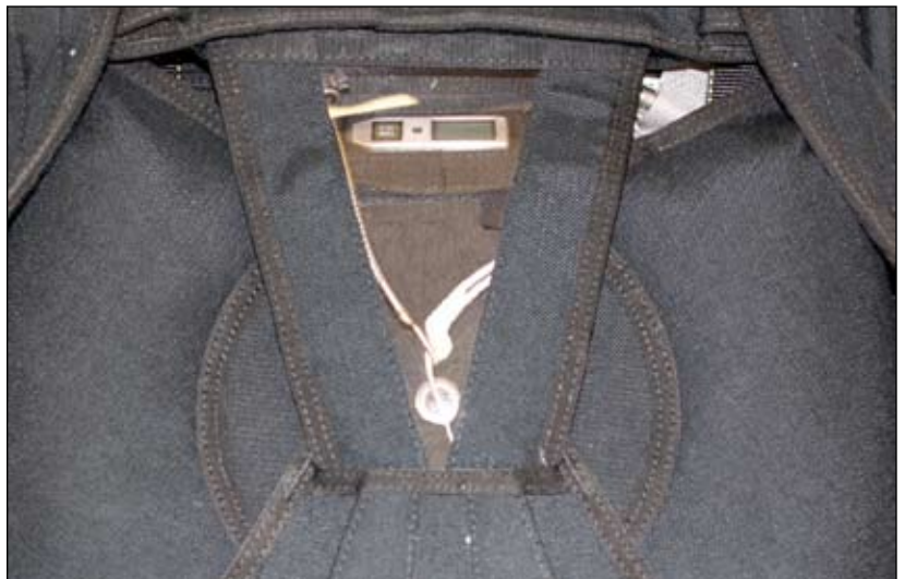
Figure 2-146. Place Pin Cover Over Flap 6
