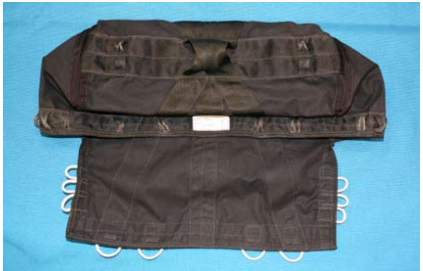
Figure 19. Outer Bag, Dual Bag Static Line
