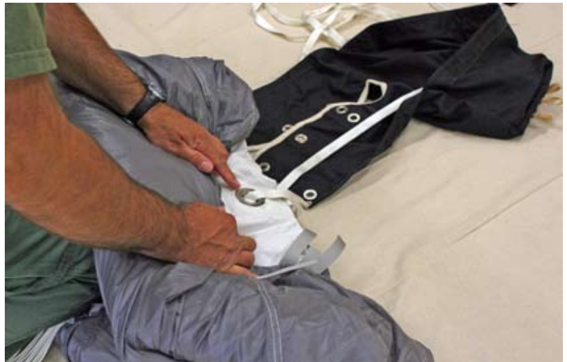
Figure 5-59. Match Parachute and Inner Bag Grommet
