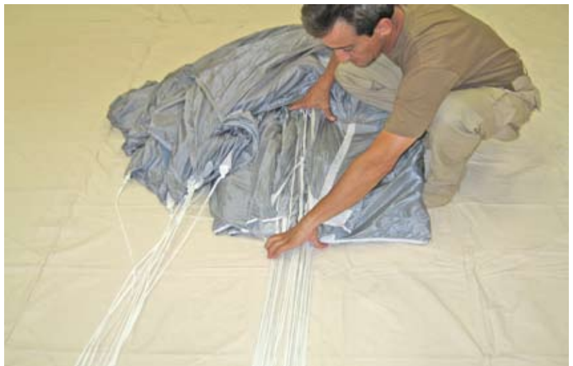
Figure 2-52. Place D Line Group Onto C Line Group
