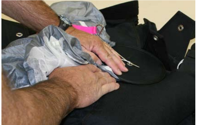
Figure 2-136. Tuck The Fabric Under The Cap
