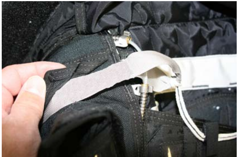
Figure 2-144. Place The Reserve Static Line
