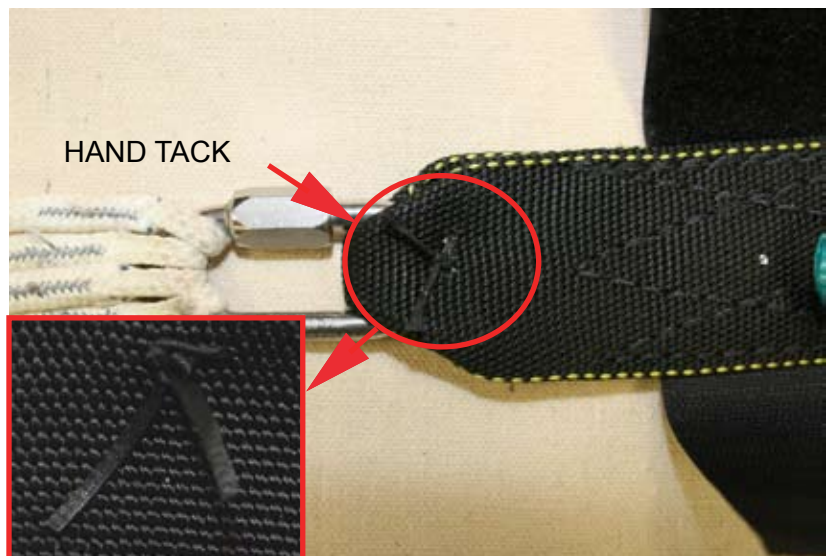
Figure 2-16. Hand Tacked Riser
