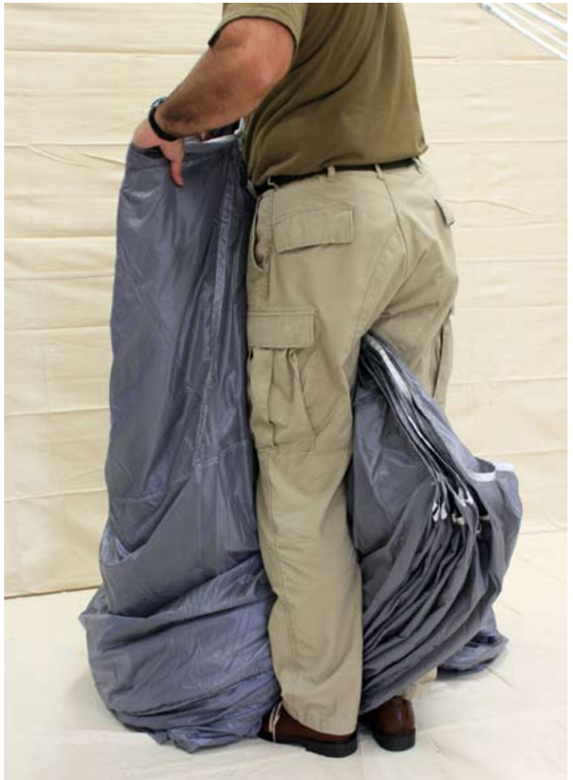
Figure 2-81. Place The Nose Between The Knees
