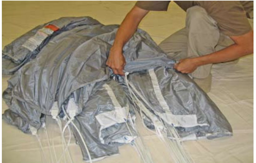
Figure 2-66. Flake The Tail
