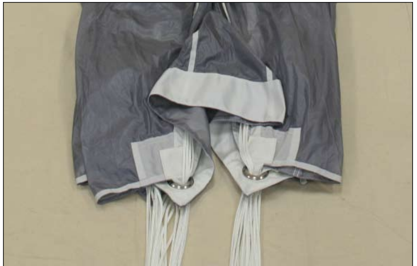
Figure 2-94. Fold Stabilizer Panels Over The Slider
