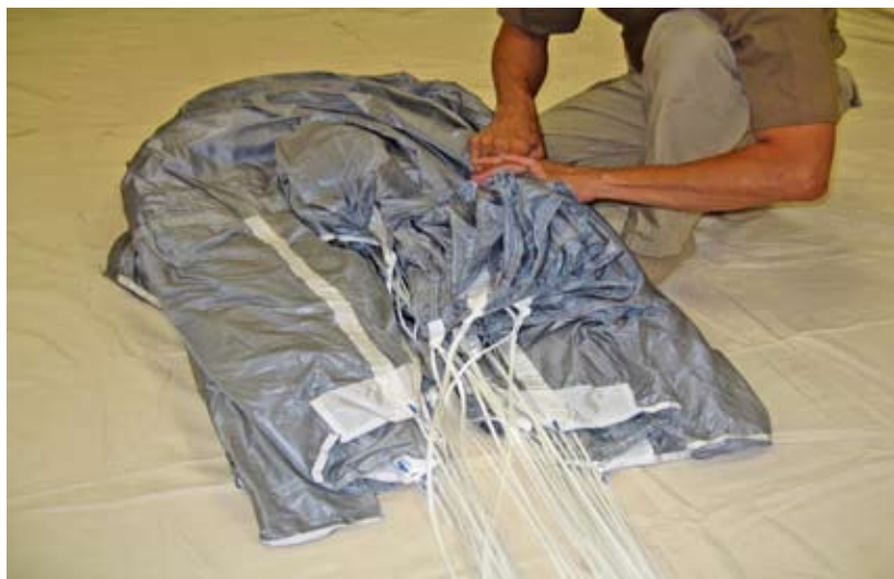
Figure 2-68. Tail Shown Flaked To One Side
