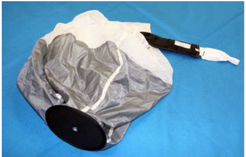
Figure 7. Pilot Chute, Reserve, W/Spring
