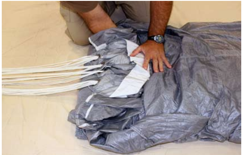
Figure 2-96. Finish The “S” Fold
