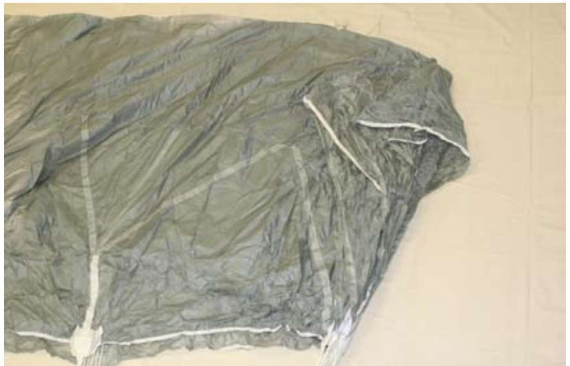
Figure 2-47. Prepare The Leading Edge
