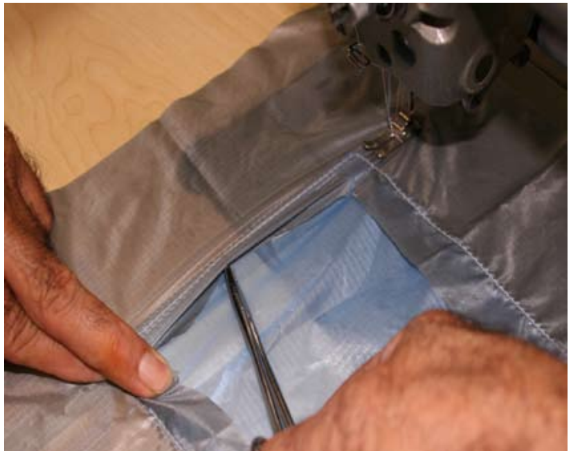
Figure 7-11. Preparing The French Seam
