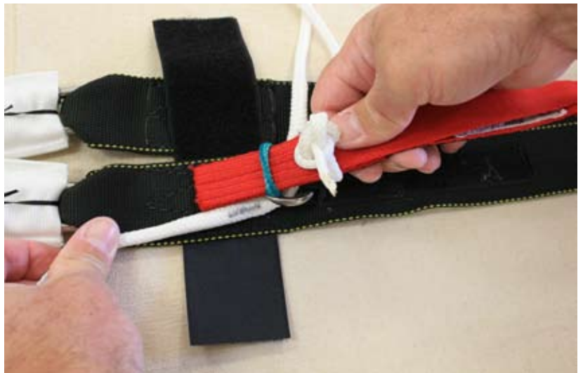
Figure 2-38. Insert Toggle Tip
