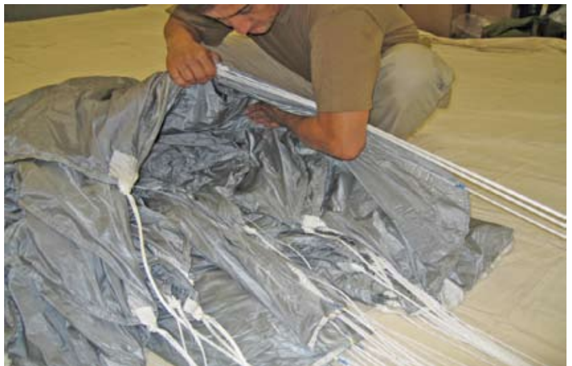
Figure 2-55. Clear Fabric Between Line Groups C & D
