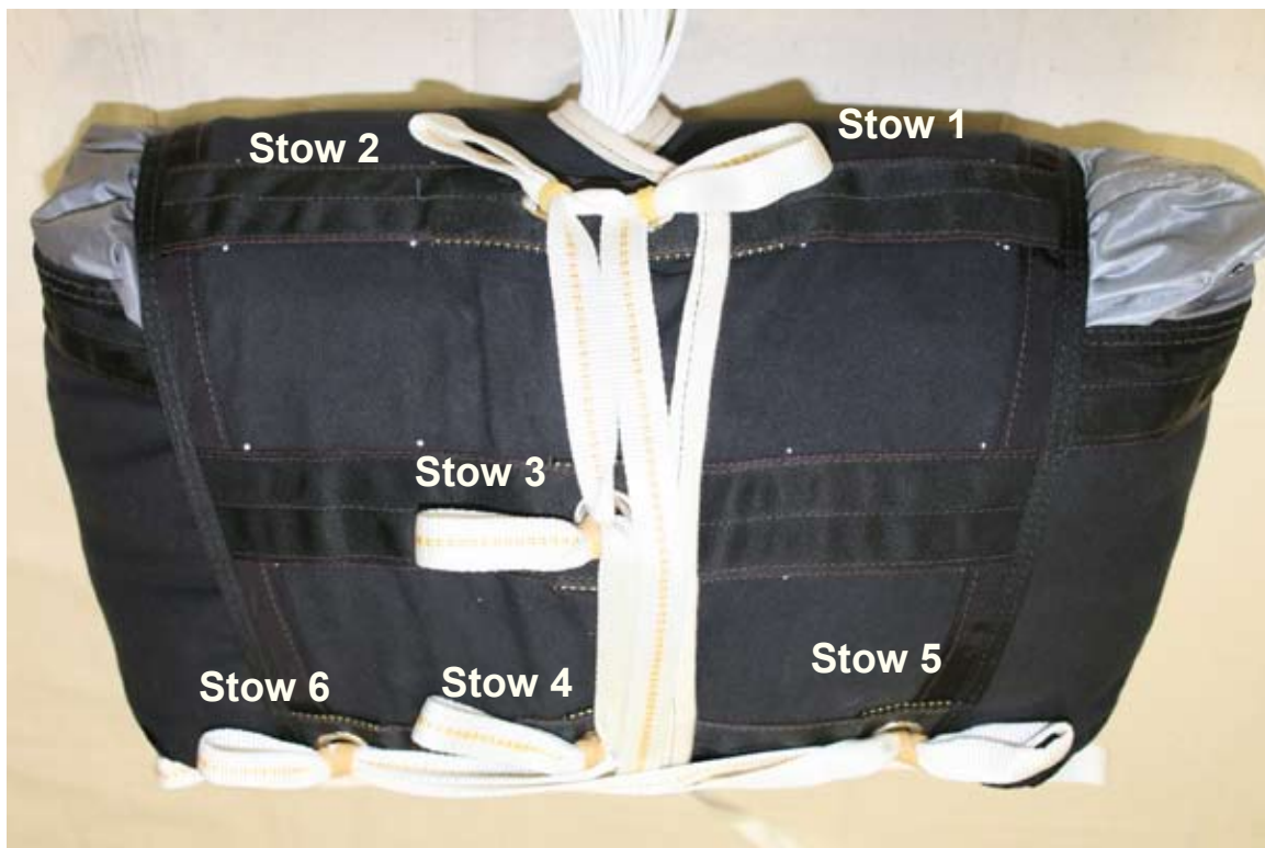
Figure 5-71. Complete The Locking Stow Sequence
