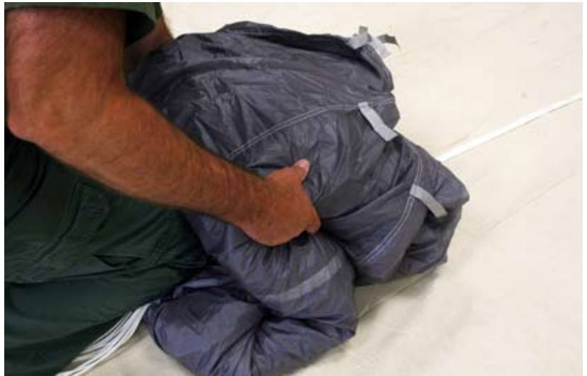
Figure 5-57. Make The Second "S" Fold
