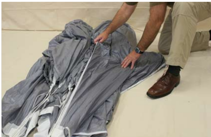
Figure 5-12. Locate The Stabilizer Panel Near The Tail Section
