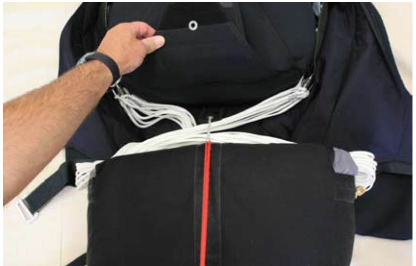
Figure 5-30. Lay The Deployment Bag Below Main Container
