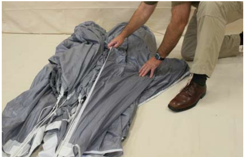
Figure 2-89. Clear The C-D Stabilizers
