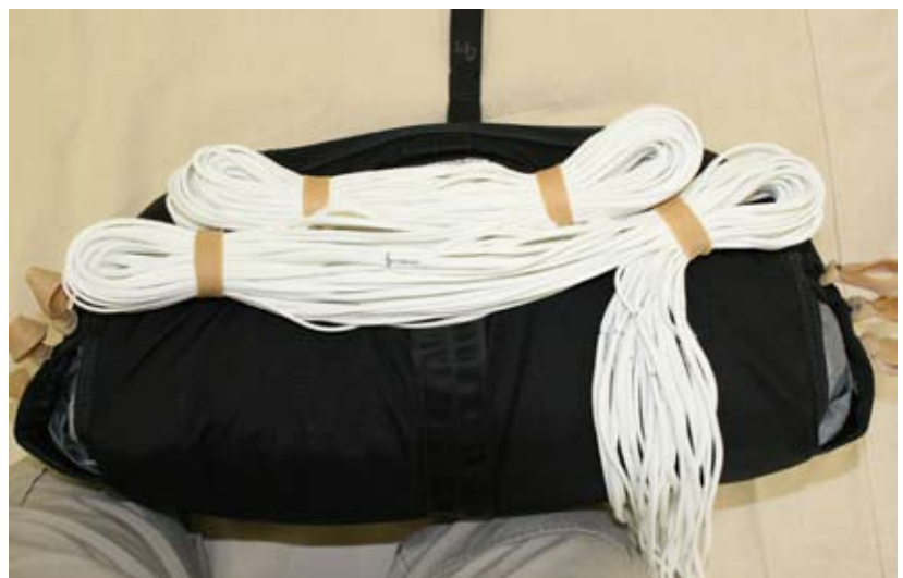
Figure 5-27. Place The Third And Fourth Locking Stow
