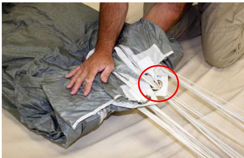
Figure 2-75. Finish The “S” Fold
