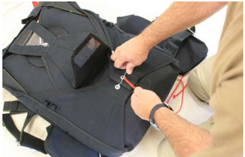
Figure 5-37. Close Flap 4 And Pin
