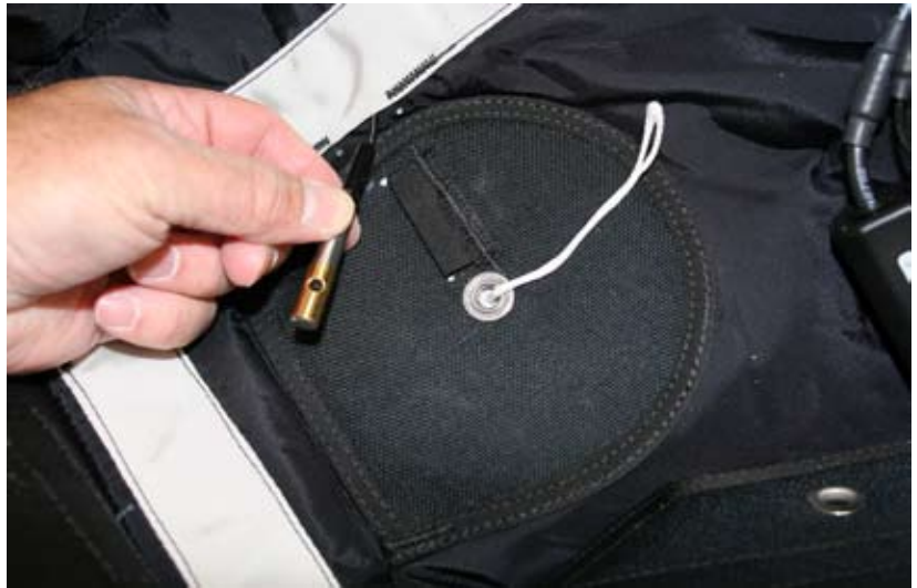
Figure 2- 5. CYPRES Cutter Routing
