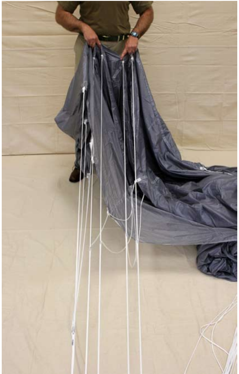
Figure 2-36. Check Steering And "D Line" Continuity
