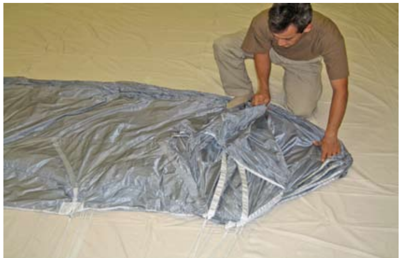
Figure 2-46. Flaking The Leading Edge
