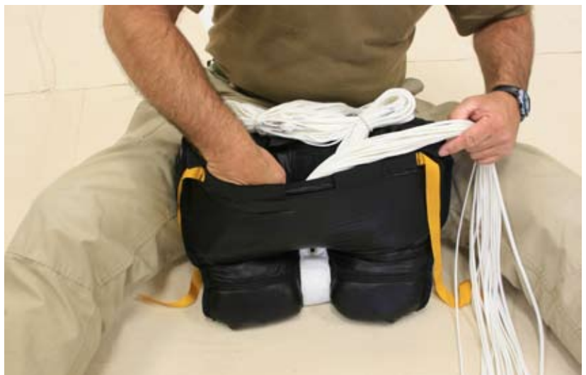
Figure 2-119. Begin Stowing The Suspension Lines
