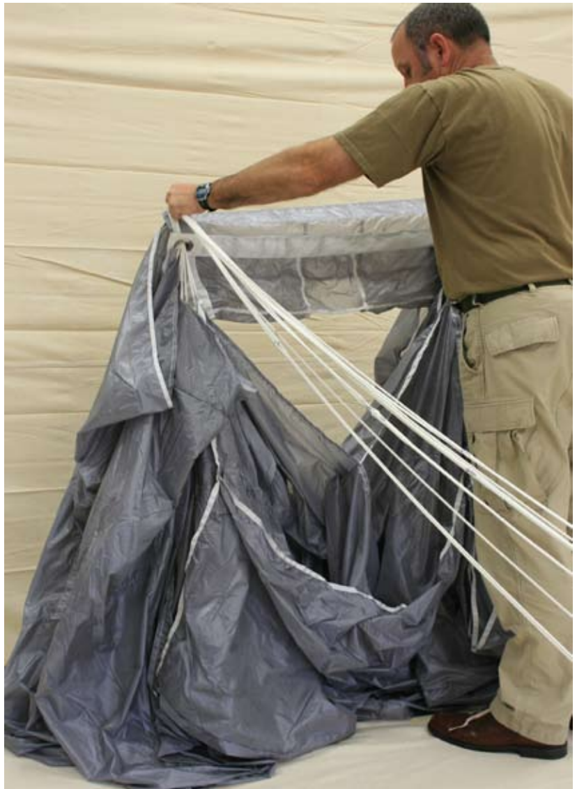
Figure 2-79. Separate The Right And Left Line Groups
