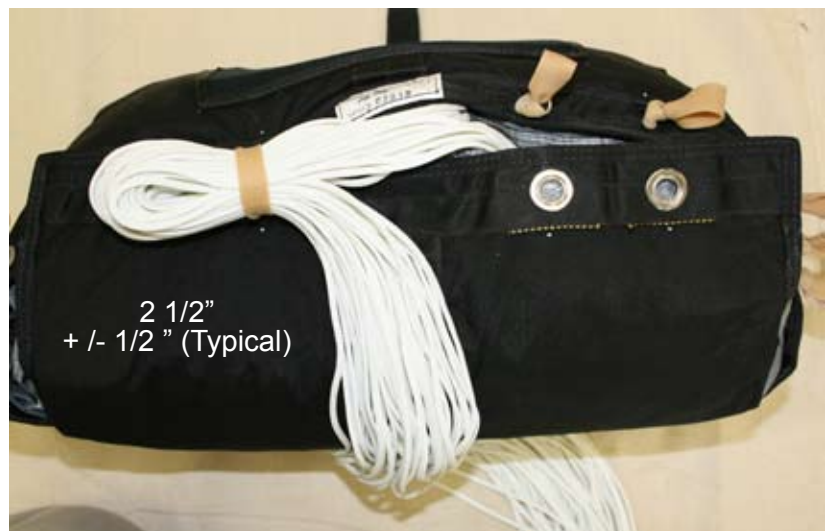
Figure 5-25. Begin Placing The Locking Stows
