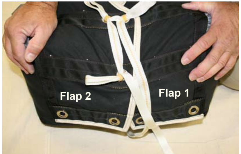
Figure 5-68. Secure Bridle Stow Number 3
