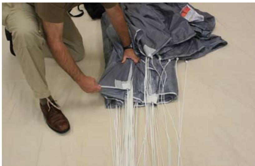
Figure 5-11. Clear The Stabilizers
