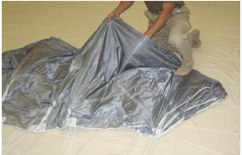
Figure 2-48. Begin Stacking The Line Groups
