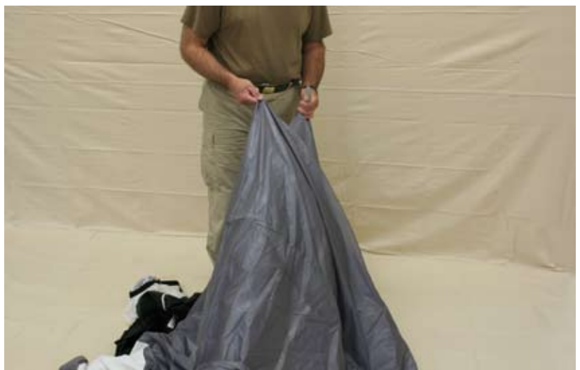
Figure 5-3. Gather Front And Rear Packing Tabs
