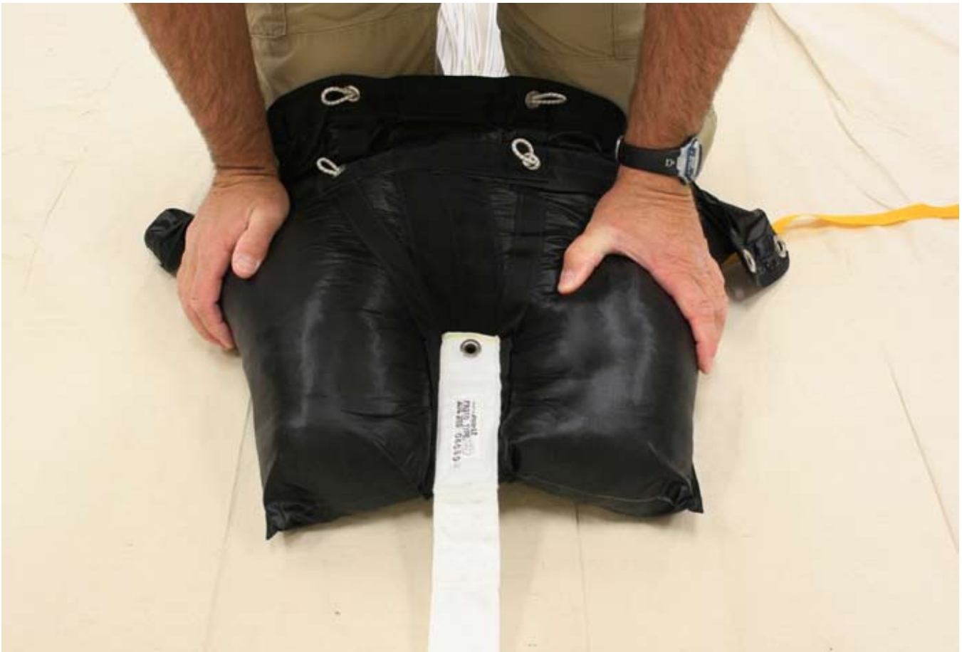
Figure 2-109. Deployment Bag Displacement Check
