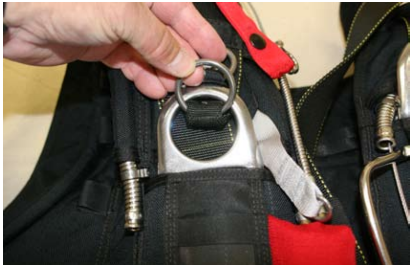
Figure 3-1. Insert Second Ring
