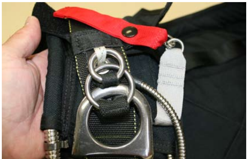
Figure 3-5. Insert The Cable Into The Retention Channel
