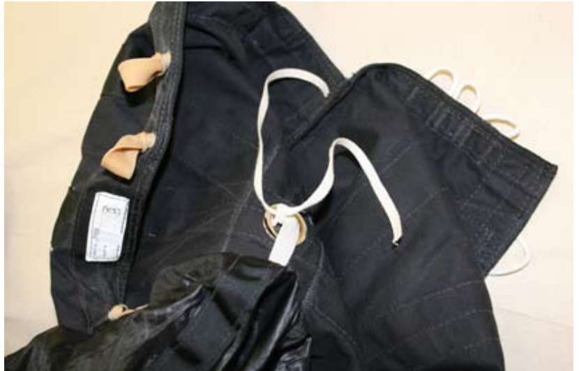
Figure 5-77. Tie The Pilot Chute To The Static Line Bag
