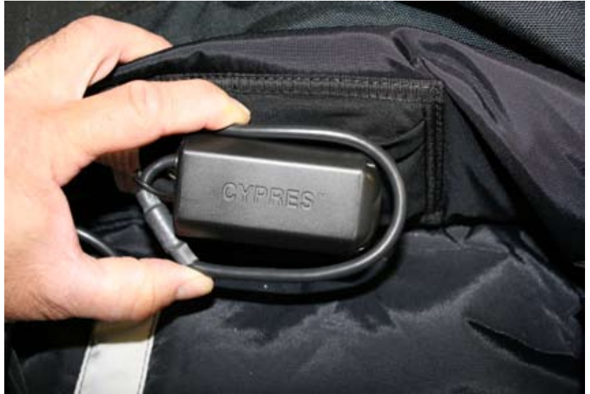
Figure 2-13. CYPRES Excess Cable Placement
