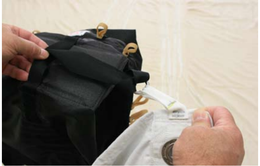
Figure 5-1. Attach the Deployment Bag To The Parachute
