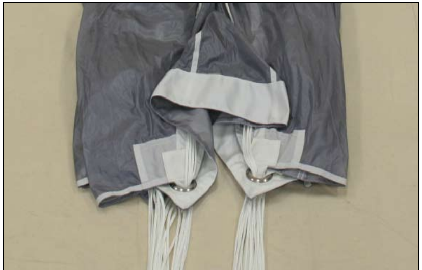
Figure 2-73. Set The Slider
