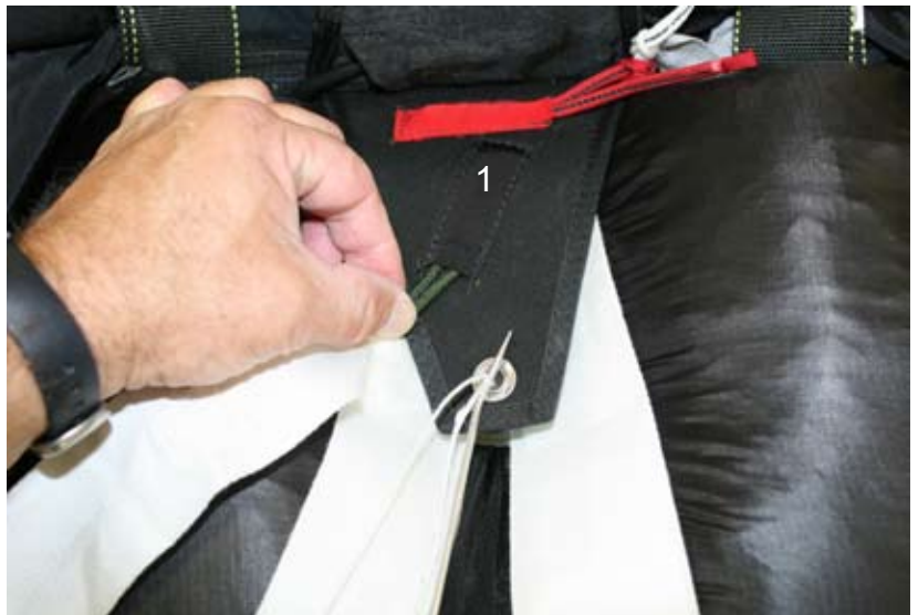
Figure 2-151. Green Loop Installation
