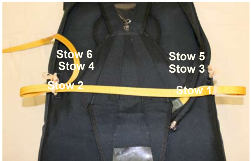
Figure 5-93. Begin To Stow The Static Line
