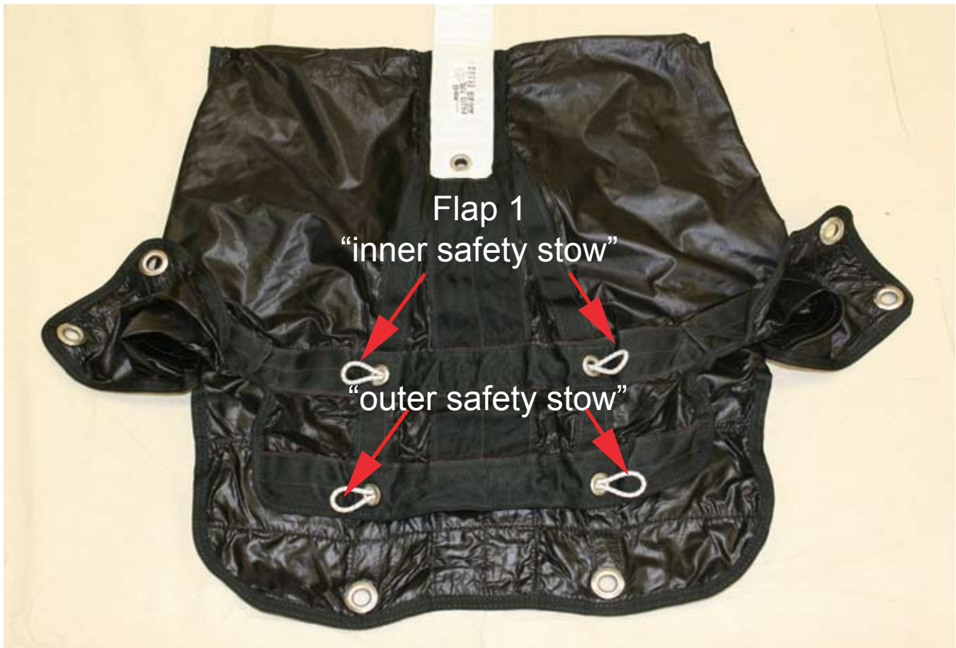
Figure 2-98. Deployment Bag Safety Stow Locations
