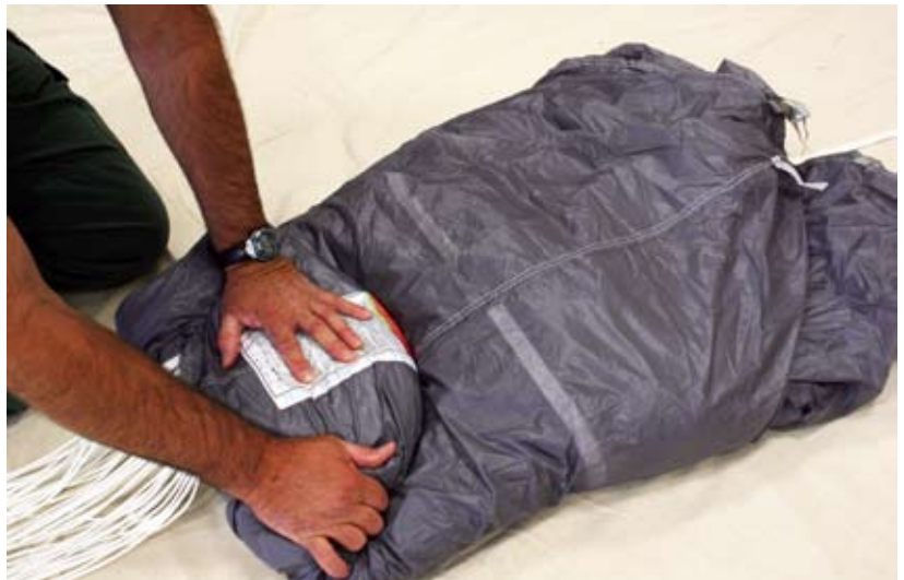
Figure 5-56. Make The First "S" Fold
