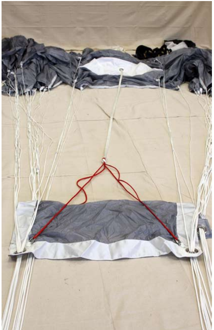
Figure 5-44. Check The Reefing Line Routing
