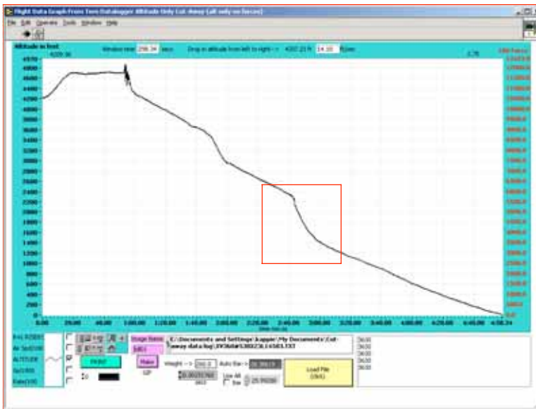
(Top) Graph of parachute flight (includes main flight, breakaway, and reserve flight). The box highlights the breakaway portion.
