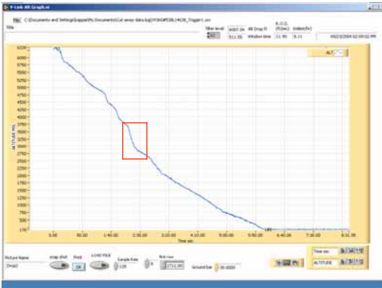
(Top) Graph of parachute flight (includes main flight, breakaway, and reserve flight). The box highlights the breakaway portion.
