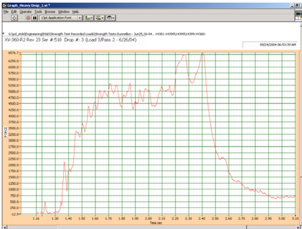
(Top) Graph of parachute deployment including approximately 10 secs of flight. The box highlights the parachute deployment.
