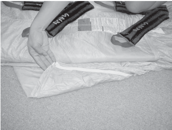
Fold the leading edge of the exposed cell openings back and parallel to the cocooned canopy.
