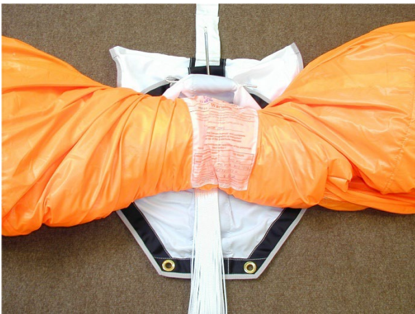
Lift up the base gently and pull the free bag underneath it. By using a T Bodkin you can make sure the base sits right at the spot where the loop will pass through later on.
