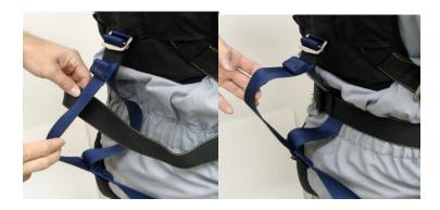
Once the horizontal back strap has been securely tightened, and all other traditional webbing adjustments have been made, the Y-Mod can then be tightened by pulling down on the excess webbing protruding from the friction adaptor located just below the harness back pad. The tightening of the Y-Mod webbing will secure the Y-Mod webbing and leg straps in place. The excess Y-Mod webbing can then be stowed under the fabric keeper.
