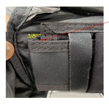
Insert tuck tab into elastic pouch so the parapack hinge lays flat. The edge of the stiffener in the tab will overhang roughly 3/8<sup>th</sup>".
