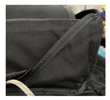
Detail of completed hand tacking with the reserve tray wrap around corner concealing the hand tacking.
