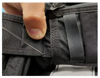
Following the same procedure to secure the bottom of the AAD tongue hinge.
