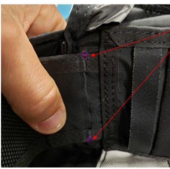
\*Detail of finished hand tacking from the inside, the hinge should lay flush and tight against the reserve tray.
