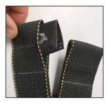
With stitching removed the Type 12 buffer can be eliminated.
